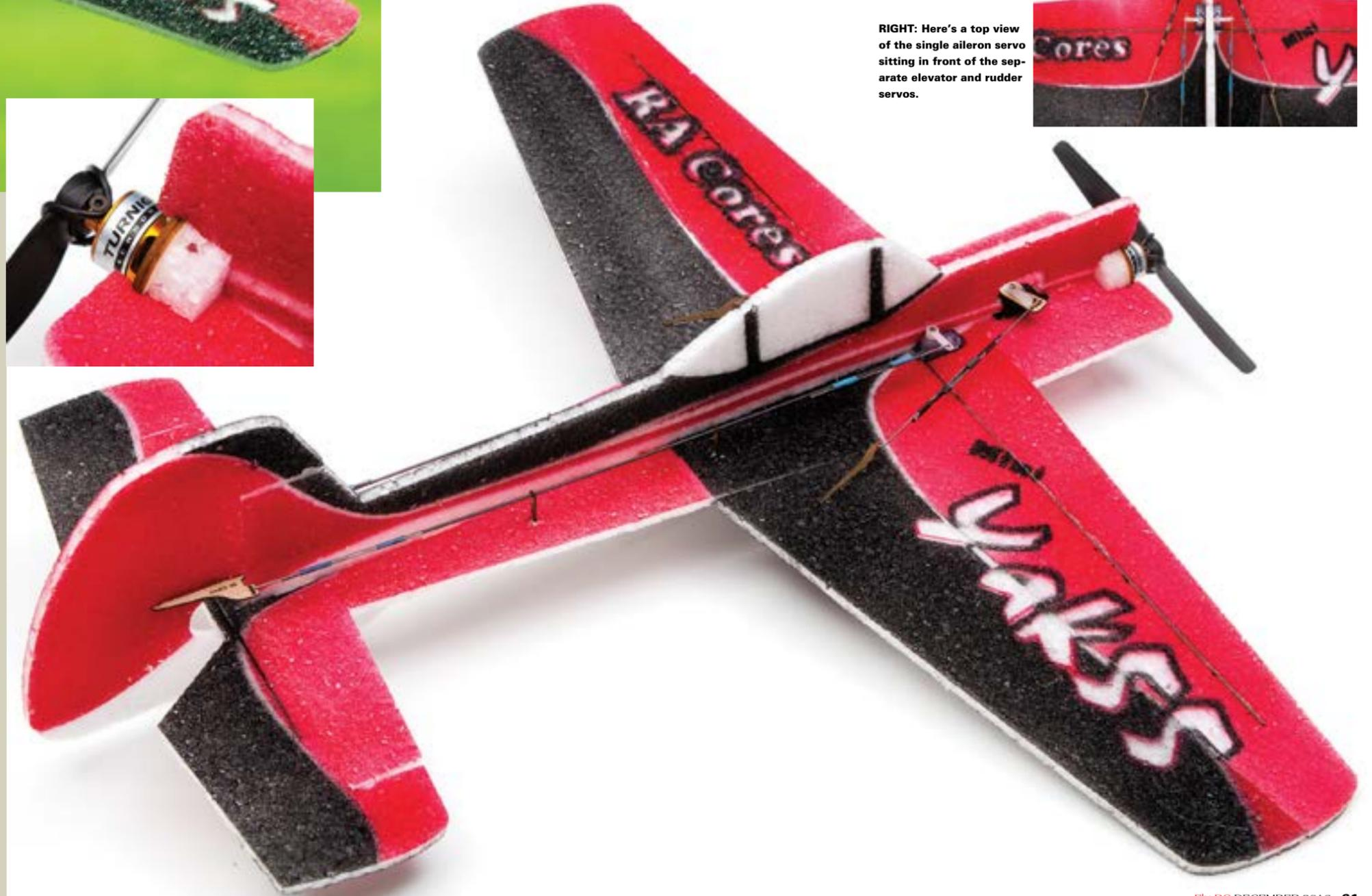
RIGHT: Here's a top view of the single aileron servo sitting in front of the separate elevator and rudder servos.
