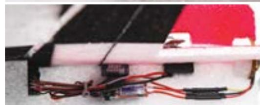
**TOP:** The Glacier 210mAh 2S flight pack sits just below the main spar on the CG. **BOTTOM:** The ESC and uncased Rx tucked into the rear fuse support.
